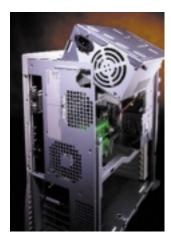
Managing service costs for your Dell system is made easier by design. The Dell Precision Workstation 220 chassis has service convenience designed in, thanks to our flip-up power supply, easy-to-access hard drive cage and the toolless entry system.
