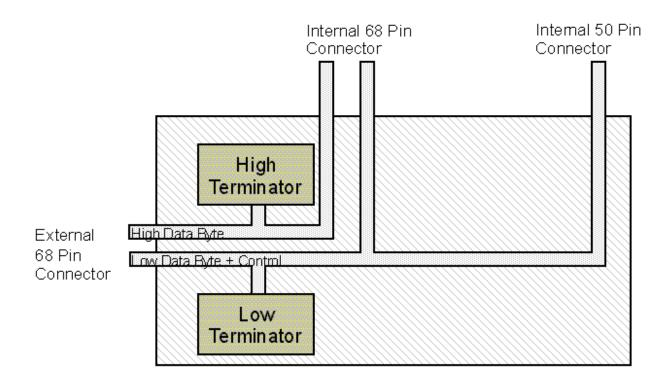
Both the PCI Fast/Wide and PCI Fast/Wide Ultra adapters contain built-in SCSI bus terminators for use when the adapter is at one physical end of the SCSI bus (i.e. you are using only internal or only external devices). The design of the controller allows for individual control of the low and high bus portions of the terminators.
