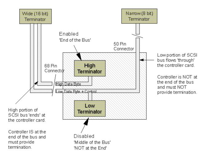
In addition to manual control, the PCI Fast/Wide Ultra adapter provides an "automatic" termination mode that properly configures the low and high bus terminators based on which connectors have SCSI cables attached. The Automatic mode should always be selected for
