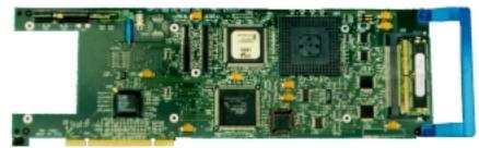
The most powerful adapter in the ARTIC family is the ARTIC960Hx PCI Adapter. This full-length, intelligent adapter is designed for use in 32-bit PCI bus host systems. Its main engine is the Intel 80960HD microprocessor which provides the performance to offload the most demanding communications and other real-time applications. On-board storage includes plug-in memory modules available in 4MB, 8MB, 16MB, and 32MB sizes.
