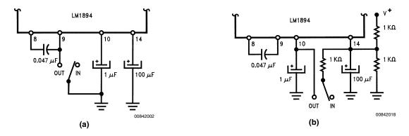
FIGURE 2. Two Methods of DNR IN/OUT Switching
