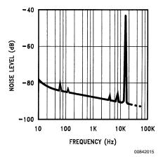
FIGURE 15. TV Noise Spectrum Level
