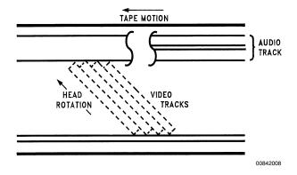
FIGURE 8. Video Magnetic Tape Format
