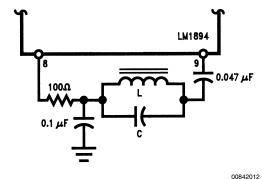
FIGURE 12. Control Path Notch Filter
