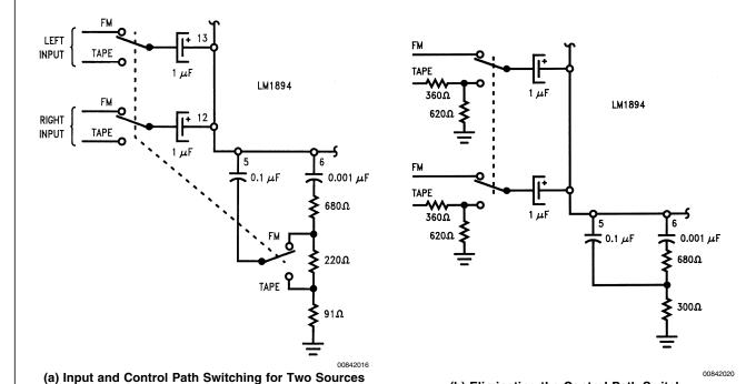
FIGURE 16. Multiple Programme Source Switching
