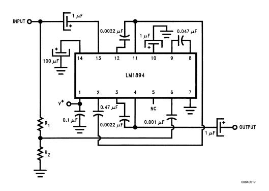
FIGURE 17. Cascading the Audio Filters of the LM1894
