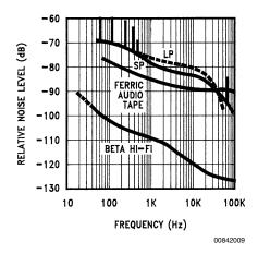
FIGURE 9. Video Tape Noise Spectrum Levels
